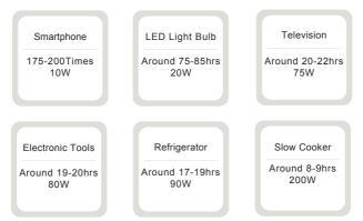
$\label{eq:2048Wh} \begin{array}{l} \times \mbox{ DOD } \times \mbox{ $\eta$} \div (\mbox{ load $W$}) = \mbox{ charging time (unit : $h$)} \\ \mbox{ Note : DOD is the battery discharge depth, $\eta$ is the local inverter efficiency, $DOD=90\%, $\eta$ = 88\%$.} \end{array}$
