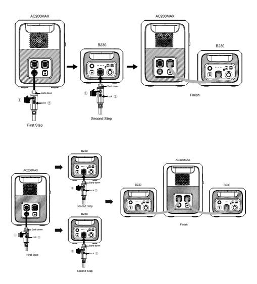
AC200MAX Capacity Extended Mode
