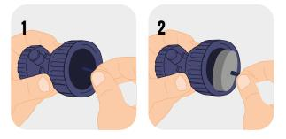
The activated carbon filter block improves the palatability of water by removing chlorine, taste and odour. Your Jerrycan will arrive without the activated carbon filter installed. See below for installation and replacement instructions.
